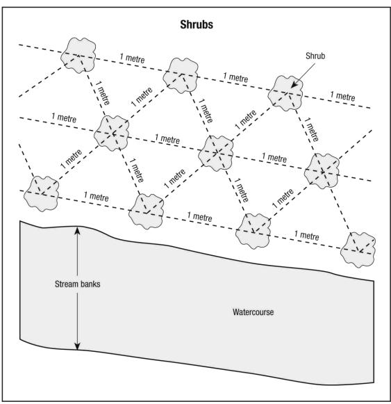
Figure 1. Conceptual drawing of typical shrub plantings (DFO, 1991).
